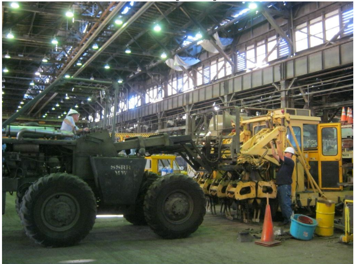
Mike H. and Brian remove the work-head assembly on the "new-old" tamper
